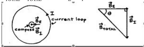
Since we wanted to determine the magnetic field of the Earth, we solved for  $B_E$ , which gave us the equation:  $B_E = B_I / \tan \theta$ .
